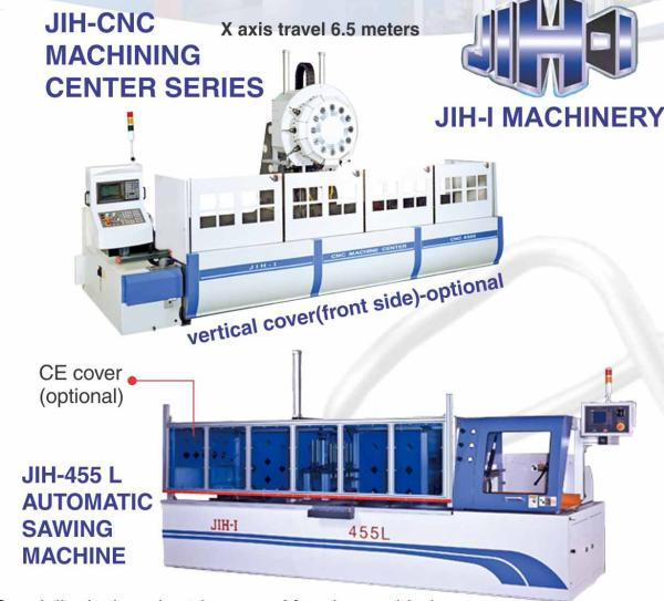
Specially designed cutting way: After the sawblade moves forward for cutting, table moves to right and left for retracting 2mm. Then the sawblade returns to its home position. This special design may avoid return-cutting, while ensuring fine surface of cut and cutting accuracy.
