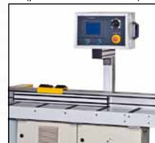
Outfeed roller table (auto- matic positioning system)
