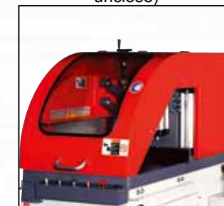
Fully enclosed guard with power off when guard opened
